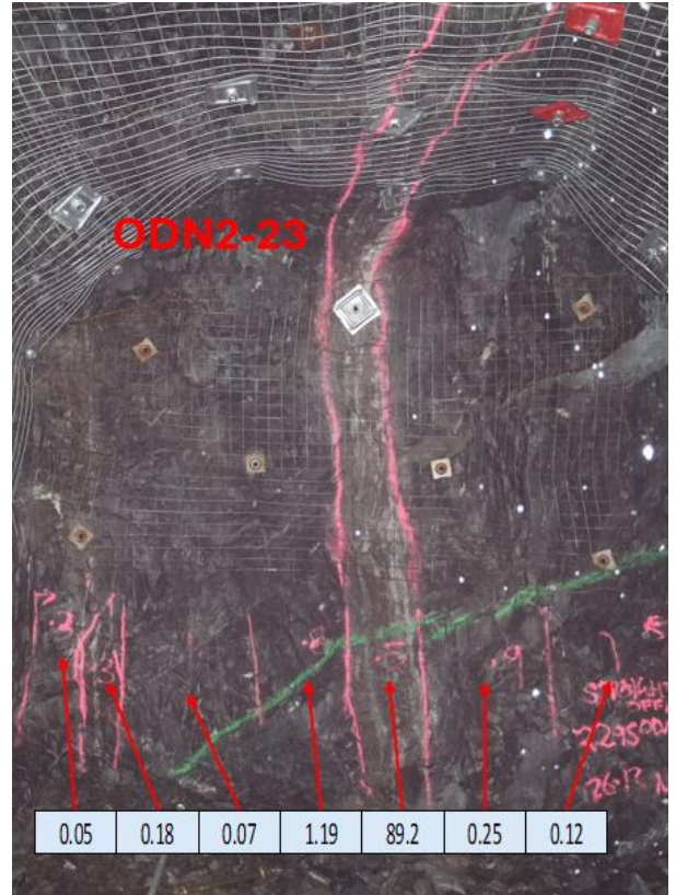
Figure 5 ODN2 23 – Face Grade 4.8m @ 9.6g/t (Uncut) Lode Grade 1.3m @ 35.0 g/t (Uncut)
