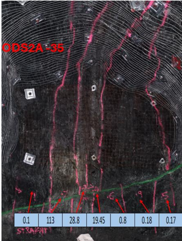
Figure 4 ODS2A 35 – Face Grade 4.4m @ 21.9g/t (Uncut) Lode Grade 1.4m @ 68.2 g/t (Uncut)
